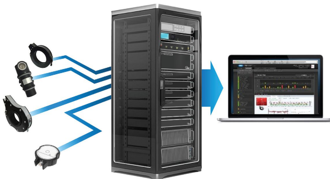
Figure 1: On-line monitoring systems consist of three functional layers: sensors, signal processing, and data interpretation.
