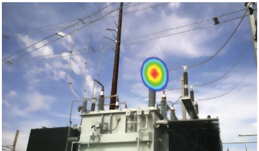
Example of Partial Discharge On or Near a Transformer Bushing IMAGE COURTESY OF FLIR
