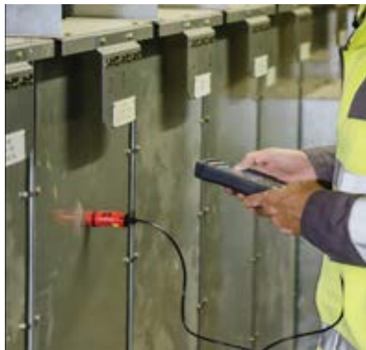
Figure 1: Contact-Type Sensor, Usually for TEV or Contact-Type Acoustic
