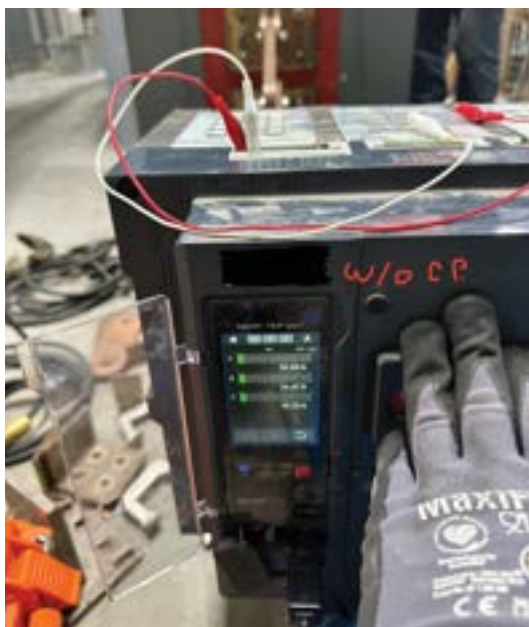
Figure 10: 30-Amp Current on All Three Phases
