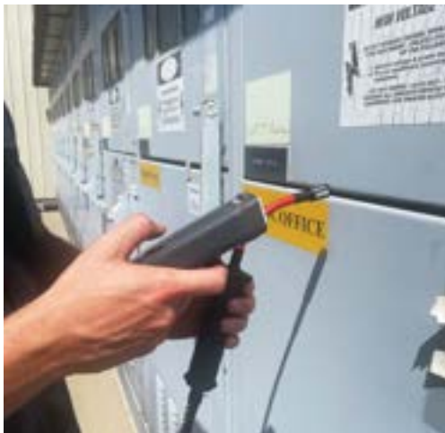
Figure 6: Acoustic PD Measurement Using an Airborne Sensor
