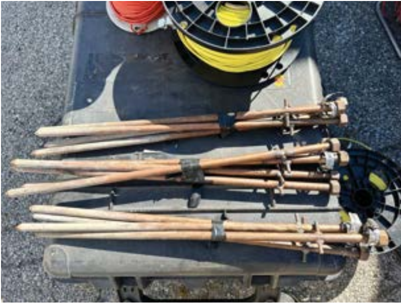
Soil resistivity testing requires sturdy, conductive probes.
