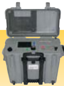
VLF 0.1 Hz @ 34 kVac Comp. control - wireless
