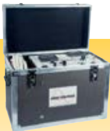
50 kVac @ 3 kVA Hipot 1 piece & w/cable output
