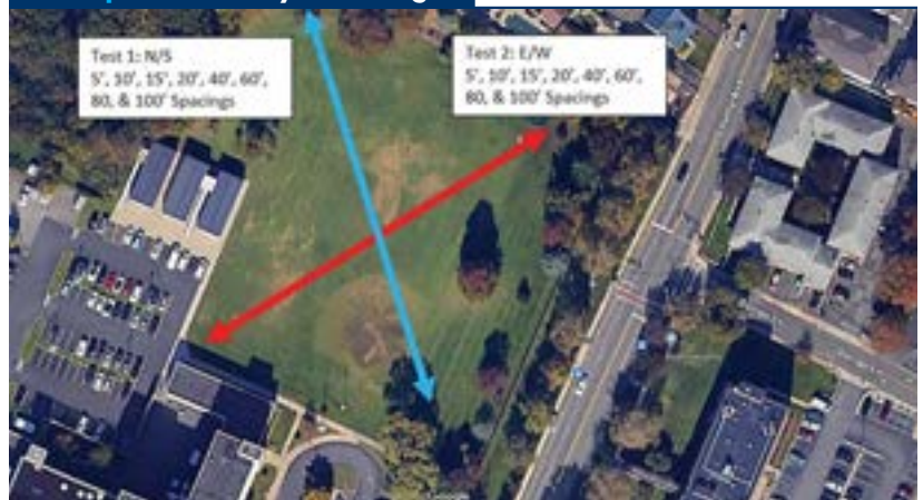
Figure 5: Results can be influenced by underground utilities and buried objects.
