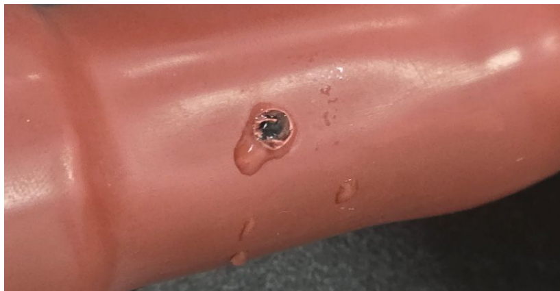
Figure 3: Artificial Pinhole Defect Introduced in Cable Jacket Near Termination
