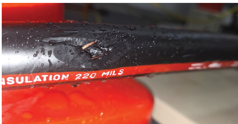
Figure 4: Deliberate Jacket Rupture with Exposed Semiconductive Layer and Applied Moisture
